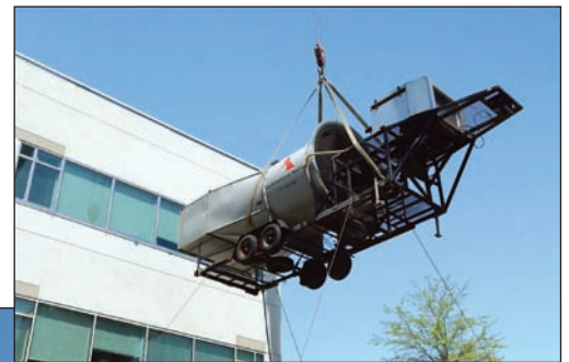
Right: Architectural Testing's Mobile Dynamic Wind Generator in Action
