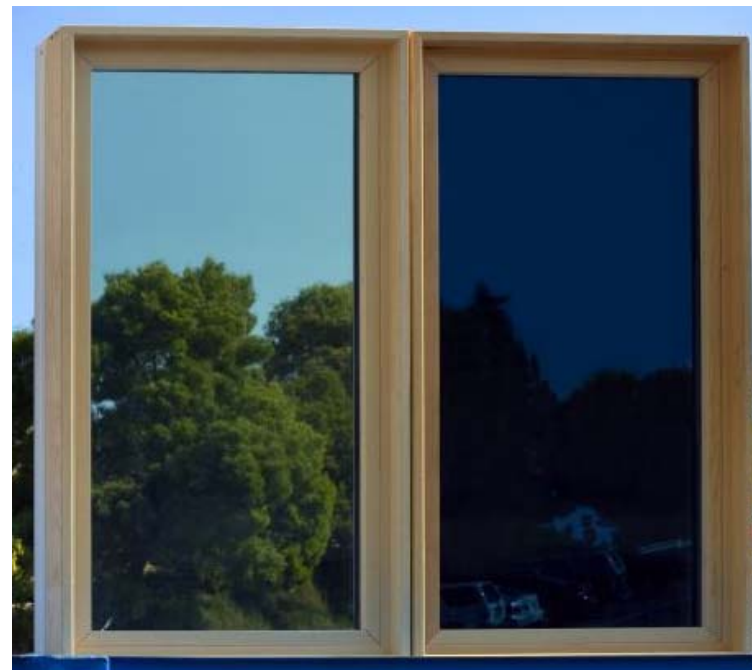
Prototype – Concept Window (Highly Insulating and Dynamic U Value 0.18 (SI U value 1.0) SHGC 0.04 – 0.34) Low cost unsealed center lite
